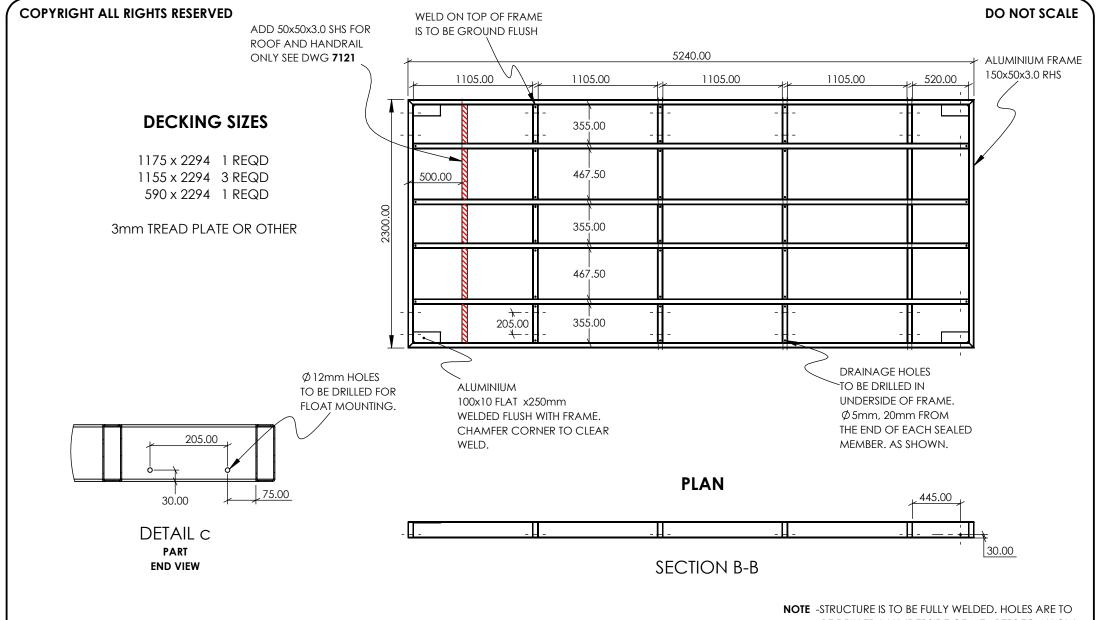
APPROX. DECK AREA - 12m<sup>2</sup> APPROX. FRAME WEIGHT - 136kg FLOATS NOT INCLUDED NOTE -STRUCTURE IS TO BE FULLY WELDED. HOLES ARE TO
